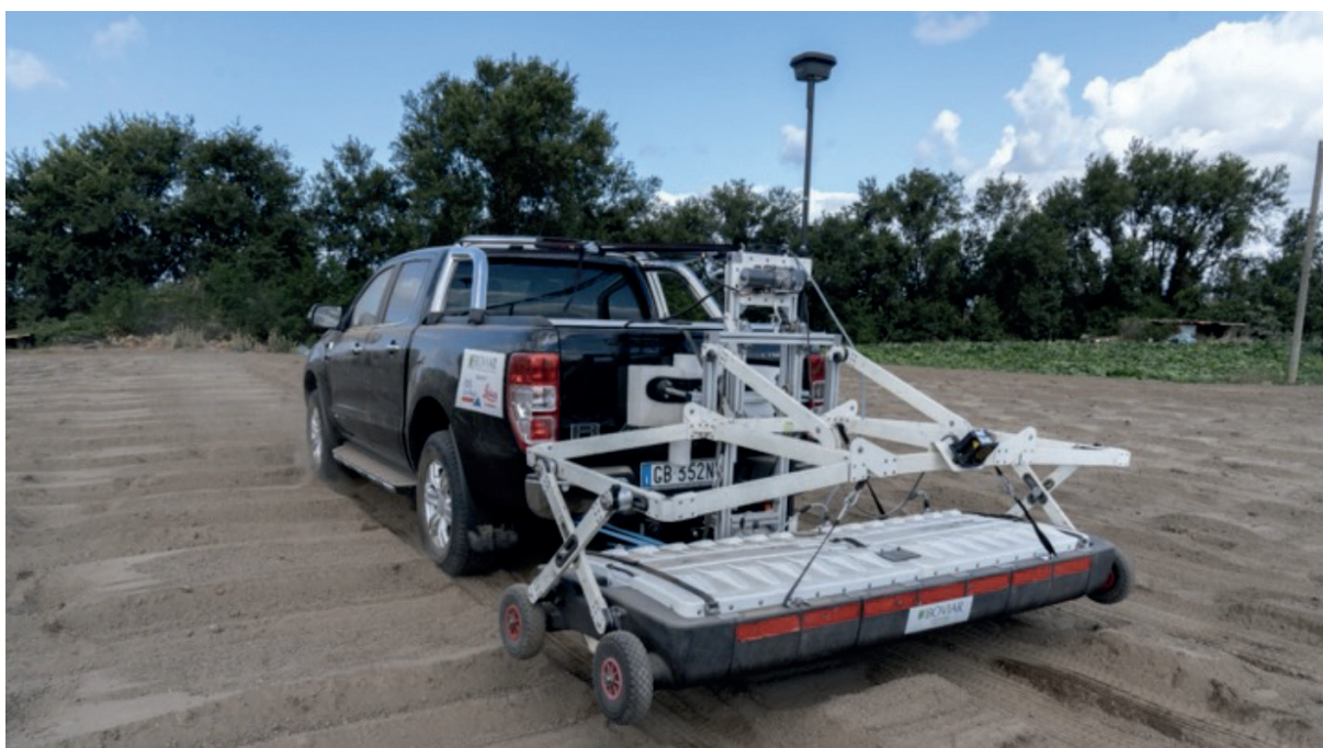
Fig. 4. Villa San Marco, indagini geofisiche 2021: area Stabia2, sistema georadar Stream X.
