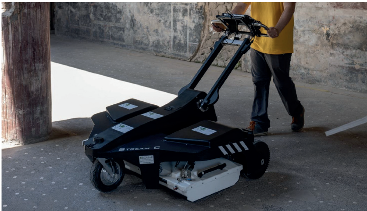
Fig. 11. Villa San Marco, indagini geofisiche 2021: area Stabia9, sistema georadar Stream C.
