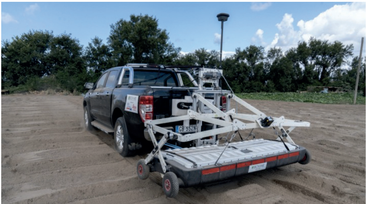
Fig. 4. Villa San Marco, indagini geofisiche 2021: area Stabia2, sistema georadar Stream X.
